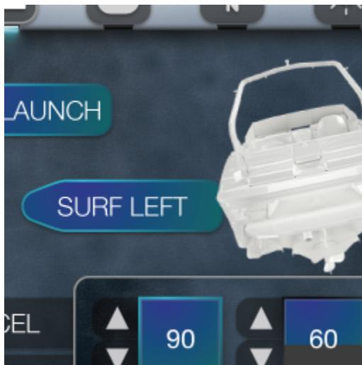
Surf Left shifts the boat on the left and enables the C Tab Setpoint (Center) and S Tab Setpoint (starboard) options.
