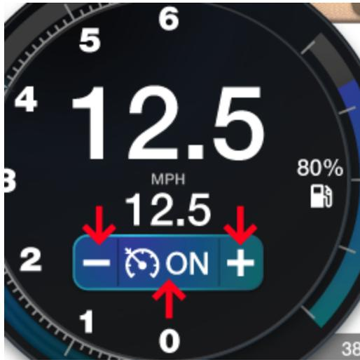
In the RPM gauge area, under MPH, tap OFF to toggle ON cruise control (the button will turn a gradient blue when active) and re-tap to deactivate cruise control. Tap the negative or plus icons to adjust the MPH speedometer.
