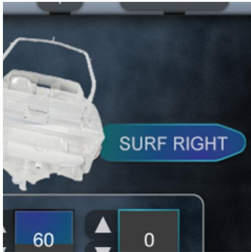
Surf Right shifts the boat on the right and enables the P Tab Setpoint (Port) C Tab Setpoint (Center) options.
