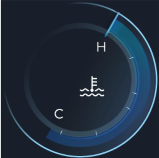
An analog engine temperature gauge. The gauge has a blue needle pointing to the 'H' (Hot) end of a scale. The center of the gauge features a thermometer icon with wavy lines below it, and the letters 'C' (Cold) and 'H' (Hot) are positioned at the bottom and top respectively. | Analog engine temperature |
