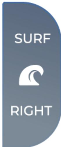
Surf Right shifts the boat on the right and enables the P Tab Setpoint (Port) C Tab Setpoint (Center) options.
